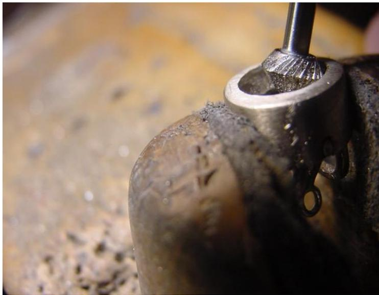
Start to make the bearing, with slight increments of cutting, so that it takes about 4-5 series of cuts to make the circle-seat. Once this is accomplished, try and place the diamond into the hole, if not, ream out the top part of the bezel, ONLY! The diamond will NOW should just fall into place inside of the hole and stay in the new made bearing. If it still doesn't, ream it open a tad more, but use a copper stone pusher to locate the stone into the seat.
