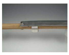
4. Position the head of the Koil Kutter over the cover plate, turn it on, and move it to the left, cutting the jump rings. Make sure to have a good grip on both the large coil holder and the Koil Kutter as there will be some resistance from the wood against the blade.
