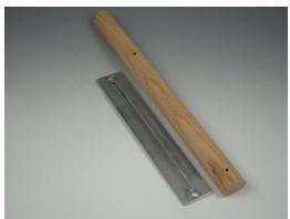
3. Drill the holes using a 9/32" drill bit.
