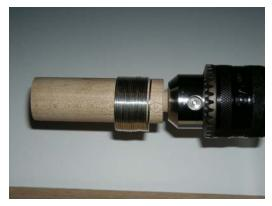
2. Slide the coil onto the large coil holder to where it will almost be in contact with the stop plate on the bottom of the cover plate.
