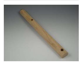
4. Turn the dowel over, and on the flat side counter sink the holes to give a little "wiggle" room to adjust the tee nuts.
