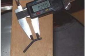
6. Place into a ring clamp or vise and cut at the line you just made, <sup>1</sup>/<sub>4</sub>" from the end, like this:
