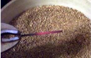
This will allow the steel to cool very slowly, perhaps as long as an hour. Be patient. I heated my piece in the Vise Grips until it was as you see in the above photo, and then plunged it into the litter. The additional heat from the pliers helped keep it from cooling too quickly. Allow to cool until you can safely touch it with your hands.
