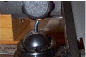
7. Now you can begin grinding this short end into the hemispherical shape needed. Use files, grinding wheels, sanding sticks, sandpaper, etc.
