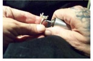
Looks a lot like a bent nail, right? You could make one from a nail, but it won't harden as well as tool steel. Before using your new rotary hammer, make absolutely *certain* that the handpiece's chuck is **<u>TIGHT!</u>** The last thing anybody wants is for one of these to go flying around the shop and break something...such as your eye.
