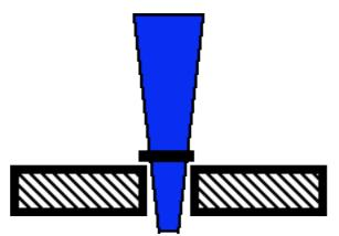
Here is a view of mandril (blue) in a hole in a bench pin (cross section of bench pin). The black band on the mandril is the bezel with the wire seat inside at bottom of bezel (can't see the seat). Tap mandril till seat is a tight fit.
