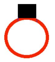
Scribe or use a fine sharple onto ring each side on the bezel. Fine blue lines. Cut vertically through the marks on the ring file the cut sides of the ring vertical.
