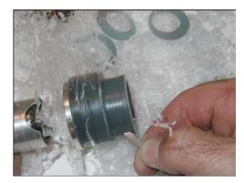
After the ring has been reduced to the desired thickness and shape, measure for the width and cut off the ring.
