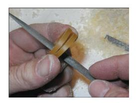
Using a 45 degree bearing bur, cut seats into the inside walls of the wax. Be cautious to keep them even and directly opposite each other.
