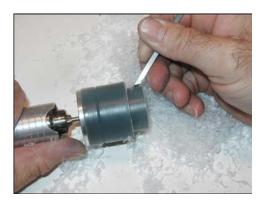
Using a finer cutting tool to add detail, start to cut and shape ridges in the wax to create a pattern around the shape.
