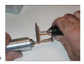
Mounting the wax is easy, just attach the table to the proper diameter mandrel and tighten the screw. Then select the wax cylinder that will best fit the shape you want to produce. There are predrilled holes in the table, one set is round holes and the other is oblong. The oblong holes are used for turning items that have an, offset finger hole. The wax has six pre-tapped holes that line up with the holes on the metal table.
