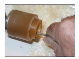
Turn the band down to a thickness of about 3mm. Next, measure and cut off a band 2mm wide. Then turn the stock edge flat and cut off another 2mm band.
