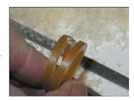
This is the completed ring. This style ring could be cast with the stone in place if desired.
