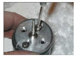
Begin to turn the outside of the ring - notice the wax appears off center to the table. Note that as the hand piece rotates, it will always retain its center point although we have changed the center point of the wax.
