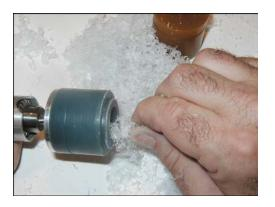
The finger hole will be centered on the wax stock. At this stage, no trimming is necessary on the exterior of the wax.
