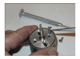
Use a tweezers and place one screw through the metal plate and into the wax, tighten the screw. Then place a screw opposite the first and tighten it also. That is all there is to mounting the wax on to the mandrel. The wax is now ready to be turned.
