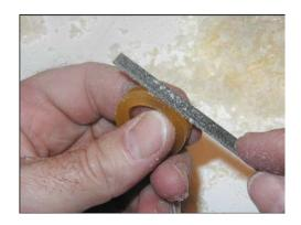
Also file the inside of the shank removing all excess wax.
