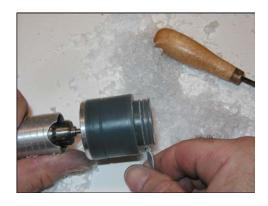
To cut the newly-created shape from the wax stock, use a scalpel blade or a flat tool and spin the hand piece to cut off the shape.
