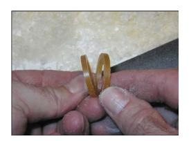
Turn the bands over keeping the ring aligned and together; place a small amount of wax on the bands to tack them together. Check the alignment of the bands and if they align properly, add more wax to complete the joint.
