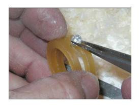
There should be some inward pressure and the stone should stay in place because of that pressure.
