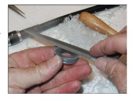
Begin to make the earring by holding the ring in one hand, and then make a saw cut through the ring as if it were going to be sized.
