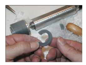
Many rings are designed thicker at the top and narrower at the bottom. This is easily created with the EZ-Lathe. First, attach the wax stock to the table using the oblong holes. Then determine the finger size; do this by removing material from the interior of the wax.
