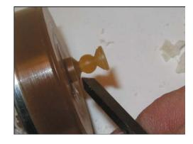
With a drill bit large enough to allow a chain to pass through, drill a hole in the center of the disk shape creating the bail opening for the chain.
