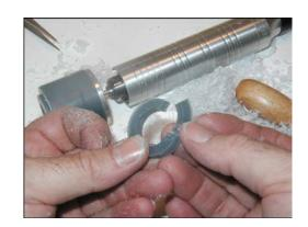
After the section has been cut away, filing will be required to smooth and shape the cut edges.
