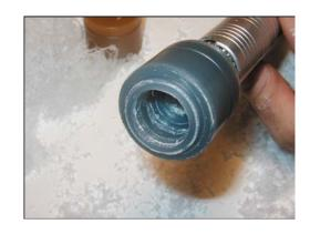
Next, you will need to take the mandrel out of the rotary hand piece. Loosen both of the screws and then shift the table to one side and retighten the screws. What has just happened is the finger hole has changed position on the table - the hole is now offset. However, by doing this, the outside of the ring can be turned on the EZ-Lathe and will result in a nicely-turned offset finger hole.
