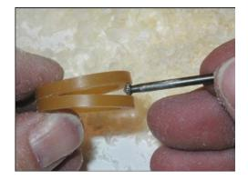
Pick up a stone and carefully place it into the stone's seat.
