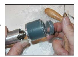
Use files to flatten and smooth the edges of the ring. This is a basic ring shape and it can be made in a matter of minutes.
