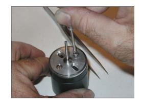
Gripping the hand piece firmly with one hand and using a cutting tool with the other hand, start rotating the hand piece. Slowly and steadily start moving the tool into the center of the wax; this results in the removal of material. This is the basic procedure to hollow a ring. Measure the inside diameter to check finger size. After the correct size has been achieved, you will be ready to turn the outside of the piece.
