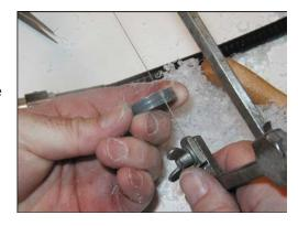
Make a second cut to remove approximately one third of the overall diameter.
