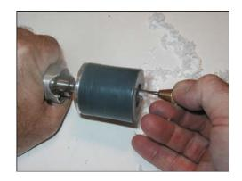
Use a cutting tool to start trimming the outside of the wax. Measure the total thickness of the carving and once the correct measurement is achieved, the wax will be ready to have details added.
