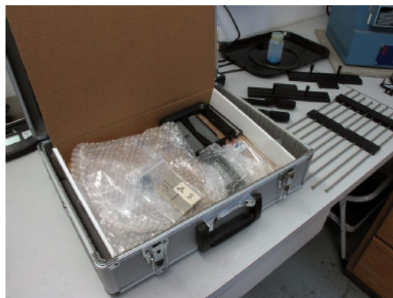
Storage case for parts, water pump hose and bottle of lubricant for engraving on glassware, straight pins/bars for holding large flat items, such as frames or plates for engraving. *Kiln shown in upper corner not included.
