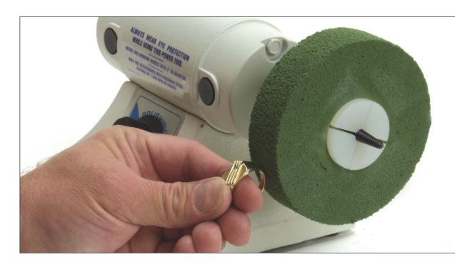
New molded wheel technology for applying semi- and final finishes on platinum, gold, titanium, precious metal clay, brass, cobalt and chrome.
