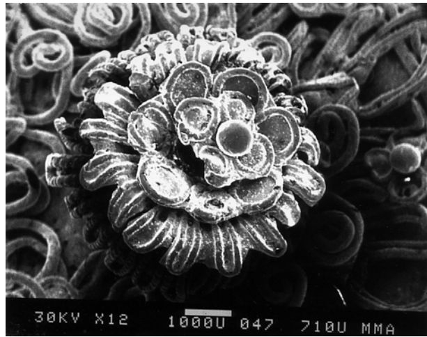
Figure 3.28. Centre rosette cap partly melted. MMA 06.1217.11 SEM by Mark Wypyski photo courtesy of the Metropolitan Museum of Art in NY.
