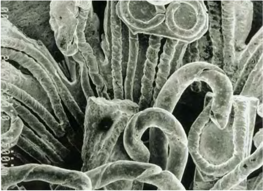
Figure 3.40. Test piece by Robert Baines Detail, Disc MMA 06.1217.11 SEM photo by Safa Shawan courtesy of RMIT.
