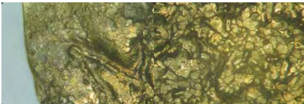
Figure 2.29,30. Test piece no.1. Square shape of the test piece with wire form is severely deformed but discernable. The sample has been heated above its solubility limit, and the grain boundaries released together cause a uniform grain growth. Stereo microscope photo by Robert Baines courtesy of the Metropolitan Museum of Art NY.
