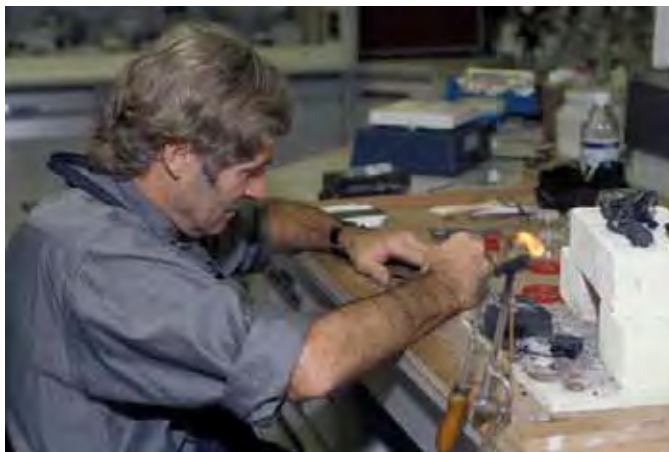
Figures 2.10-12. A laboratory workstation in the chemistry laboratory was established at The Sherman Fairchild Center for Object Conservation at the Metropolitan Museum of Art in New York. Preparation of gold samples, wire making with chisel and wood block, granules and the fire joining of gold samples. photo courtesy of the Metropolitan Museum of Art in NY.
