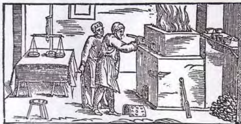
Figure 13. An assaying laboratory, showing balances, muffle furnace for cupeling, ingot mould, etc.
