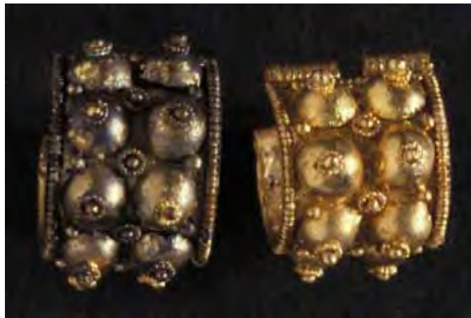
Figure 3.22. Gold laboratory reproduction by Robert Baines of gold a baule ear ornament MMA. 95.15.146 Oxide on surface as an outcome of the copper salt joining process on the left and the other boiled in salt and vinegar. Photo by Robert Baines courtesy of the Metropolitan Museum of Art in NY.
