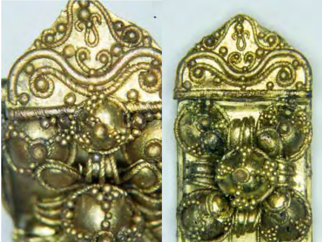
Figures 3.7,8. Gold laboratory reproduction by Robert Baines of gold a baule ear ornament MMA. 95. 15.138. Oxide on surface as an outcome of the copper salt joining process. Grooved wire having the appearance of twisted on the pediment. Stereo microscope photo by Robert Baines courtesy of the Metropolitan Museum in NY.
