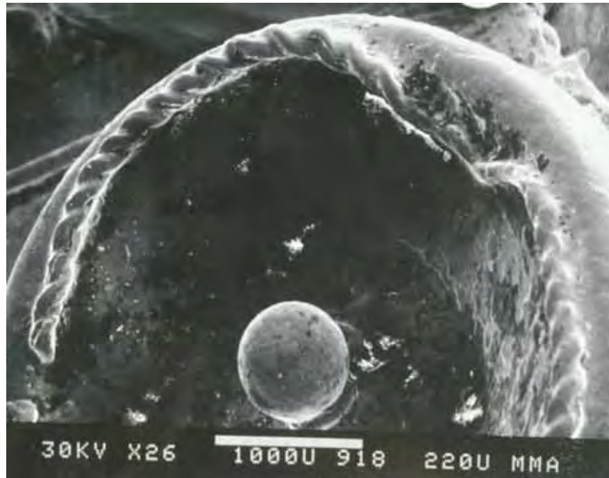
Figure 2.19. Detail. Gold Etruscan a baule ear ornament. The Metropolitan Museum of Art New York. Roger's Fund, 95.15.141, 142. SEM photograph of grain growth on concave bowls and substrate of the pediment. SEM photo courtesy of the Metropolitan Museum of Art in NY.
