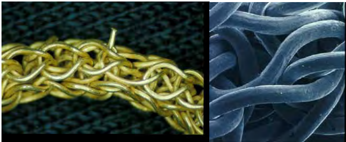
Figures 1.4,5. Wire working in a loop and loop chain of a fake that has the same stylistic mistakes as figures 5,6. Clearly the chain is not made by the same goldsmith. Photo by Gail Spring and SEM image by Robert Baines and Barry Smith courtesy of RMIT.
