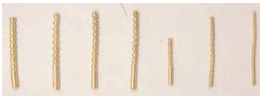
Figure 2.38. Test Pieces by Robert Baines. Beaded wire made using the Organarium
