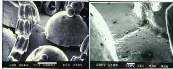
Figures 2.1,2. Etruscan gold a baule ear ornament MMA 95.15.139, fourth century BC. The grooved folded strip has lifted to reveal preliminary marking out on the substrate by the goldsmith. SEM image courtesy of the Metropolitan Museum of Art in NY.
