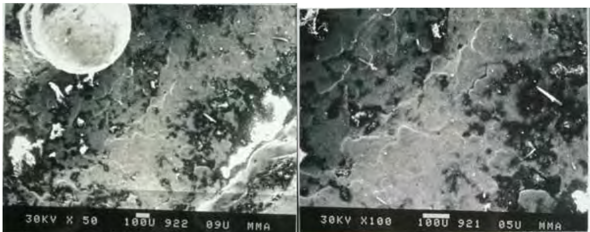
Figures 2.20,21. Detail. Gold Etruscan a baule ear ornament., The Metropolitan Museum of Art New York. Roger's Fund, 95.15.141,142. SEM photograph of grain growth on concave bowls and substrate of the pediment. The orientations of the crystal axes in the different grains are grouped closely about a common mean value. 31 There is a macroscopic segregation of equiaxed solidification. SEM photo courtesy of the Metropolitan Museum of Art NY.
