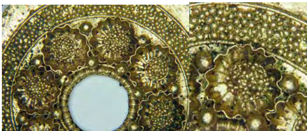
Figure 2.8,9. Test piece by Robert Baines. Hollow ball construction using copper salt diffusion joining. Stereo microscope photo by Robert Baines courtesy of the Metropolitan Museum of Art in NY.
