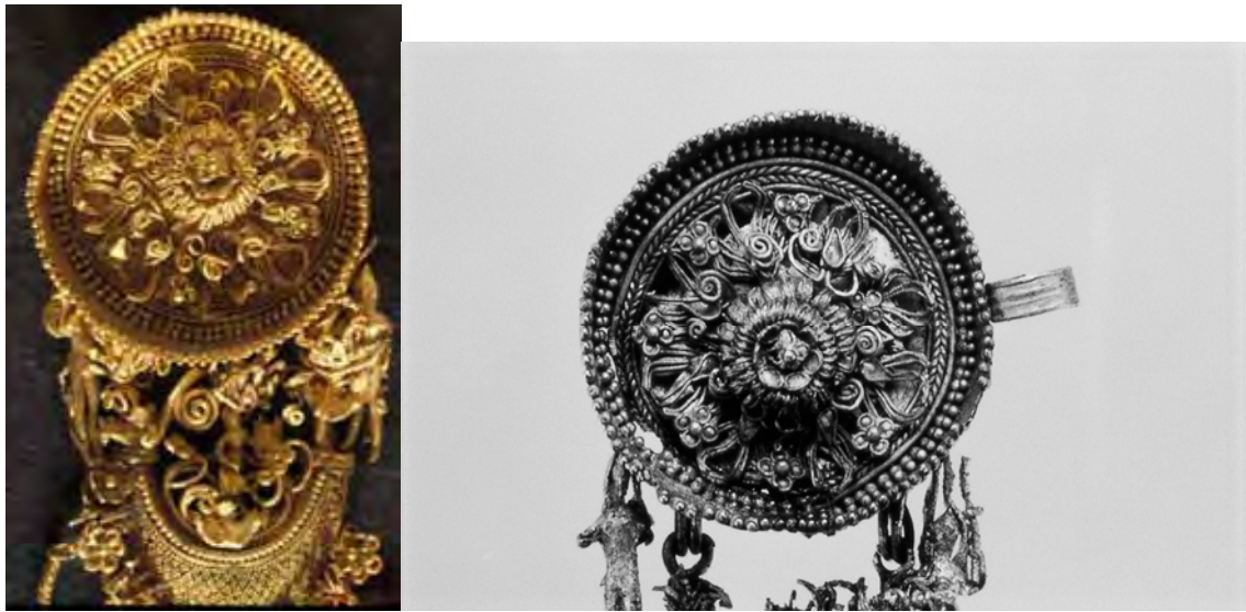
Figures 3.25,26. Detail. A swaged gold hair ring has fused to the wall of the disc as a consequence of high temperatures within a reducing atmosphere. MMA 06.1217.12. photo by Robert Baines courtesy of the Metropolitan Museum of Art in NY.
