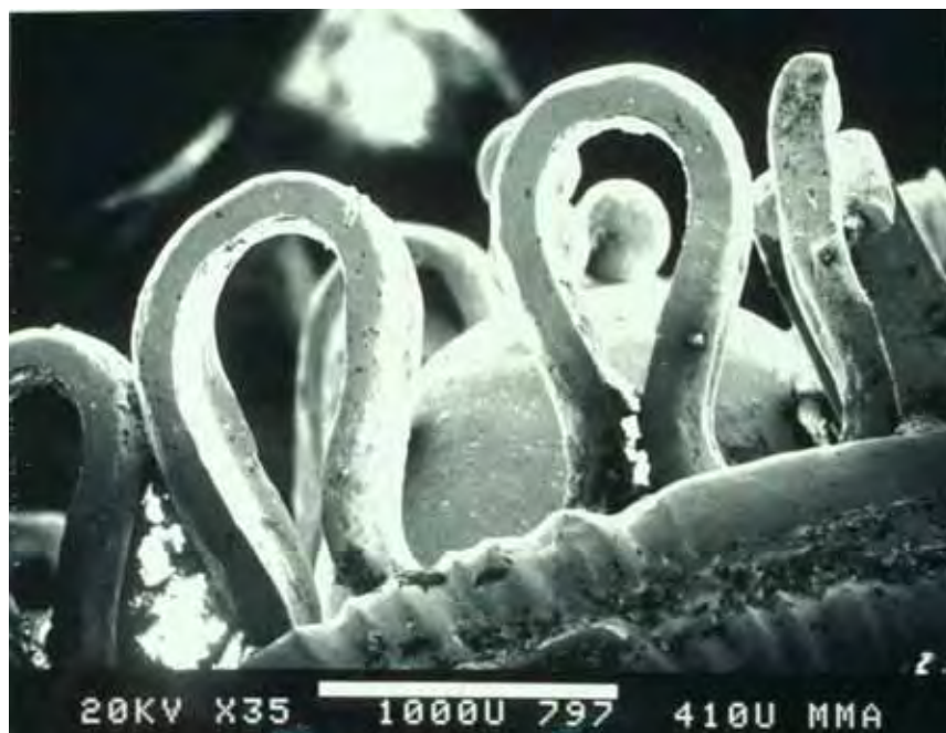
Figure 3.18. Gold a baule ear ornament MMA. 95.15.139 Grooved folded strip. SEM by Mark Wypyski photo courtesy of the Metropolitan Museum of Art in NY.
