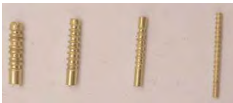
Figure 2.37. Test Pieces by Robert Baines. Spool wire made using the Organarium .
