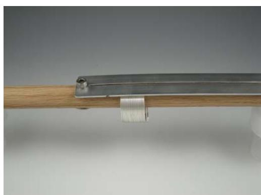
4. Position the head of the Koil Kutter over the cover plate, turn it on, and move it to the left, cutting the jump rings. Make sure to have a good grip on both the large coil holder and the Koil Kutter as there will be some resistance from the wood against the blade.
