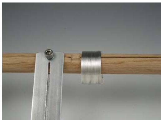
3. Apply a little burr life to the top of the coil. Attach the other end of the cover plate, and tighten the screws making sure the coil is against the stop plate.
