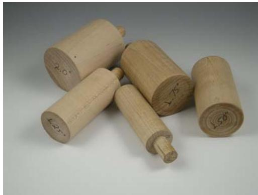
I had a friend make a set of large mandrels on his wood lathe that fit in my winder, but just using dowels and hand winding the coil will also work.
