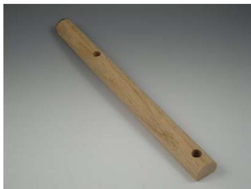
4. Turn the dowel over, and on the flat side counter sink the holes to give a little "wiggle" room to adjust the tee nuts.
