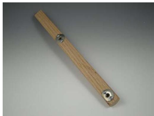
7. Turn the dowel in the side and mark where the little stop plate is on the bottom of the cover plate. Unscrew the cover plate and cut away enough material with the wood rasp to allow the cover plate to make full contact with the dowel.
